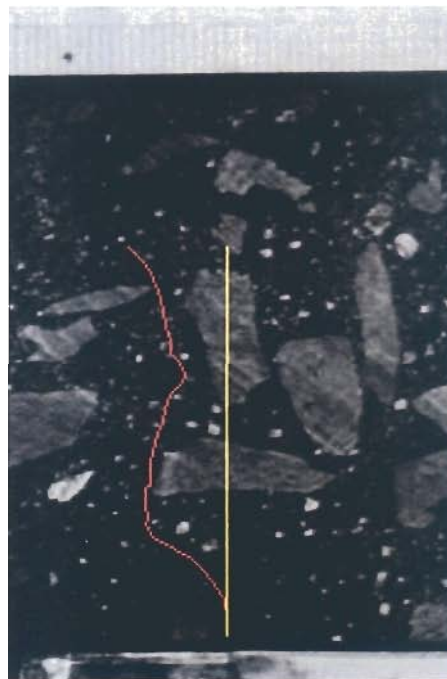
Color Plate III (See page 26, Plate 7) Electronically superimposed crack on unpainted beam – specimen HRA5HO2
